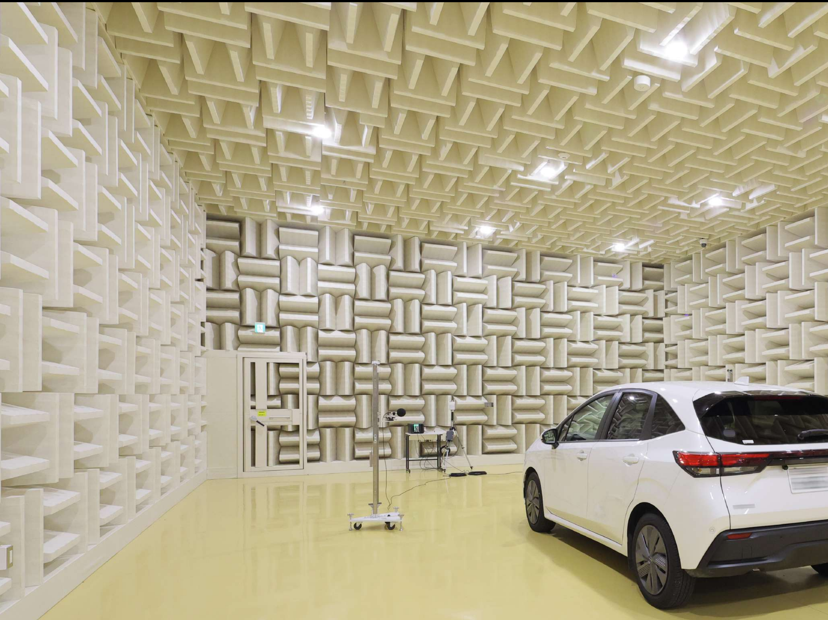
National traffic safety and environment laboratory. Semi-anechoic chamber for conducting commissioned acoustic tests on vehicles at a public institution in Japan.
