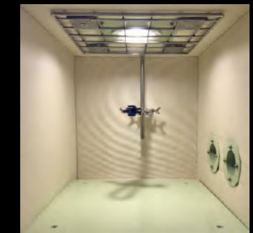
Lighting, Clamp for microphone, mesh ceiling, unburnable interior materials
